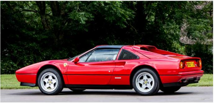
The Ferrari 308 was superseded by the mechanically similar but larger engined 328 GTB in 1985. By increasing both bore and stroke, the quattrovalvole engine's capacity was raised to 3,186cc which, together with a higher compression ratio, revised pistons and an improved Marelli engine management system, lifted maximum power to 270bhp at 7,000rpm. Top speed was raised to within a whisker of 160mph (258km/h) with the sprint to 60mph covered in 5.5 seconds.
